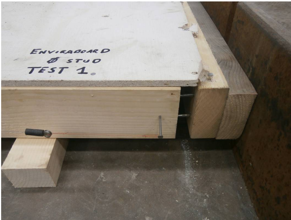
Plate 1 – Typical Mode of Failure after 0 kN Vertical Top Load Tests
