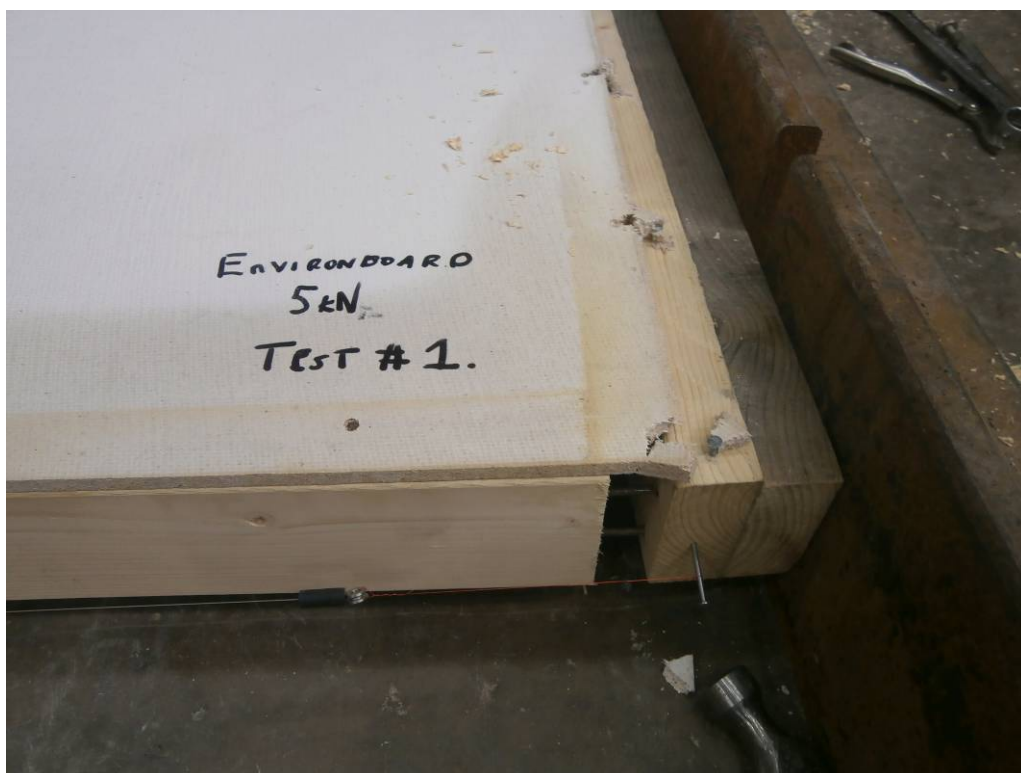
Plate 2 – Typical Mode of Failure after 5 kN Vertical Top Load Tests
